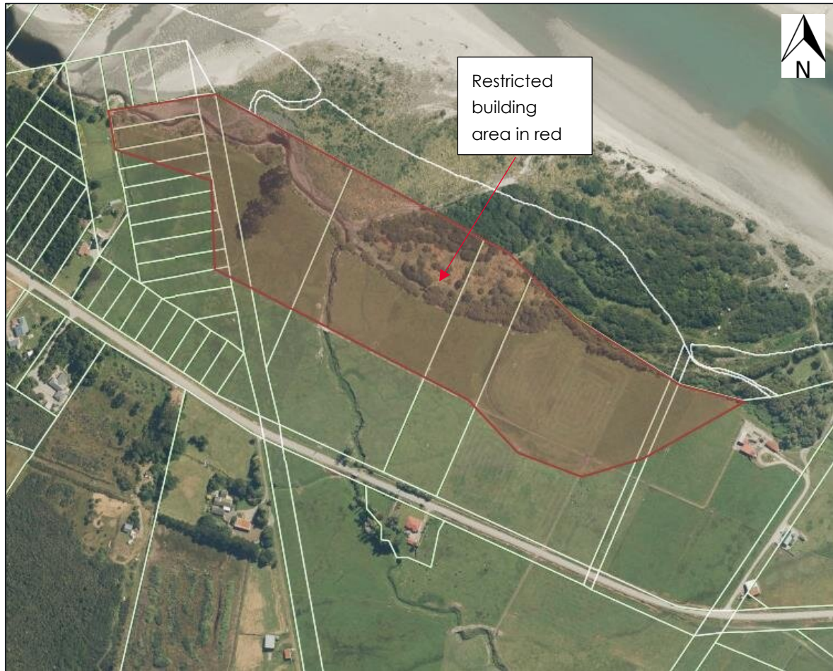
Figure 8. Area to be restricted from building (Eliot Sinclair 2022)
